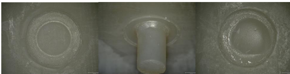
Figure 3. Overview of failure types: Adhesive between the substrate and the luting composite ( left ), cohesive within the luting composite ( middle ), and cohesive within the 3D printed resin ( right ).
