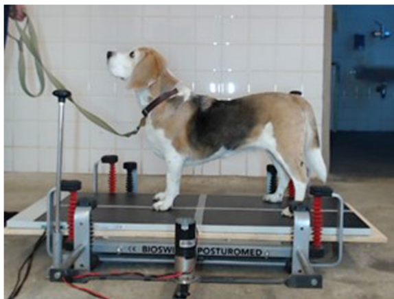
Fig. 3 Standing Position on the modified Posturomed platform: The dogs were positioned as straight as possible longitudinally on the platform with each paw placed in its corresponding quadrant
