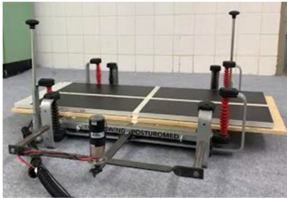
Fig. 2 Modified canine Posturomed platform
