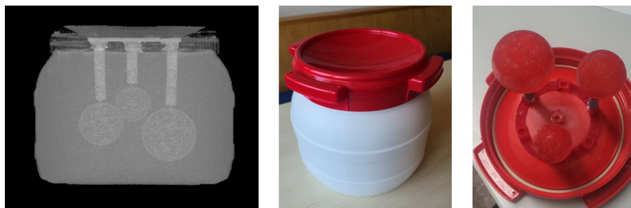
Fig. 1 CT (left), photographs of the self-designed phantom (center) and the three fillable spheres (right)
