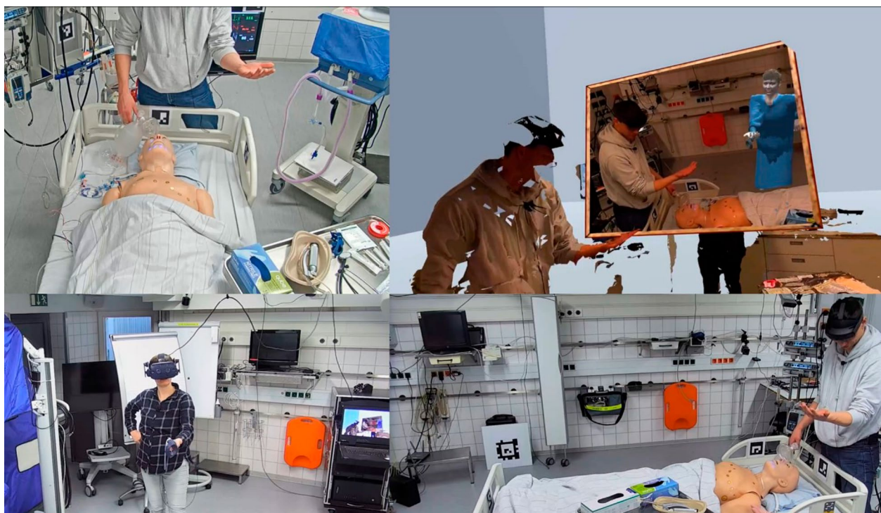
Fig. 3 Four perspectives showing the interaction possibilities. The remote expert (bottom left) and the avatar (top right) demonstrate a gesture, which is copied by the AR HMD user
