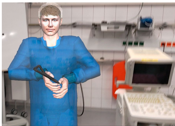
Fig. 2 HoloLens 2 AR HMD view: the avatar representing the remote expert
