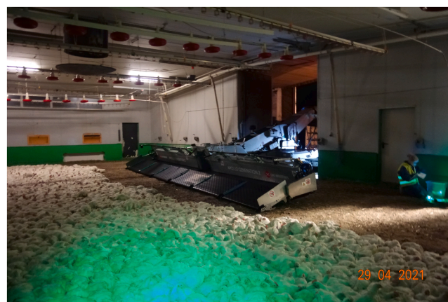
Fig. 1. Modified version of the Apollo Generation 2 loading machine (CMC Industries-Ciemmeclabria, Cazzago S. Martino, Italy).
