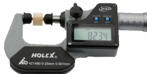
Figure 2. Digital micrometer screw gauge and representative specimen.
