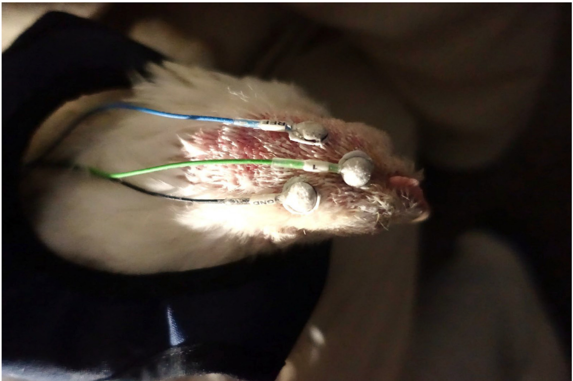
Fig. 4. The localization of attached surface electrodes. An EEG adhesive paste was used between the electrodes and the scalp, sample animal: genotype Ross 308 of light conventional fattening program.
