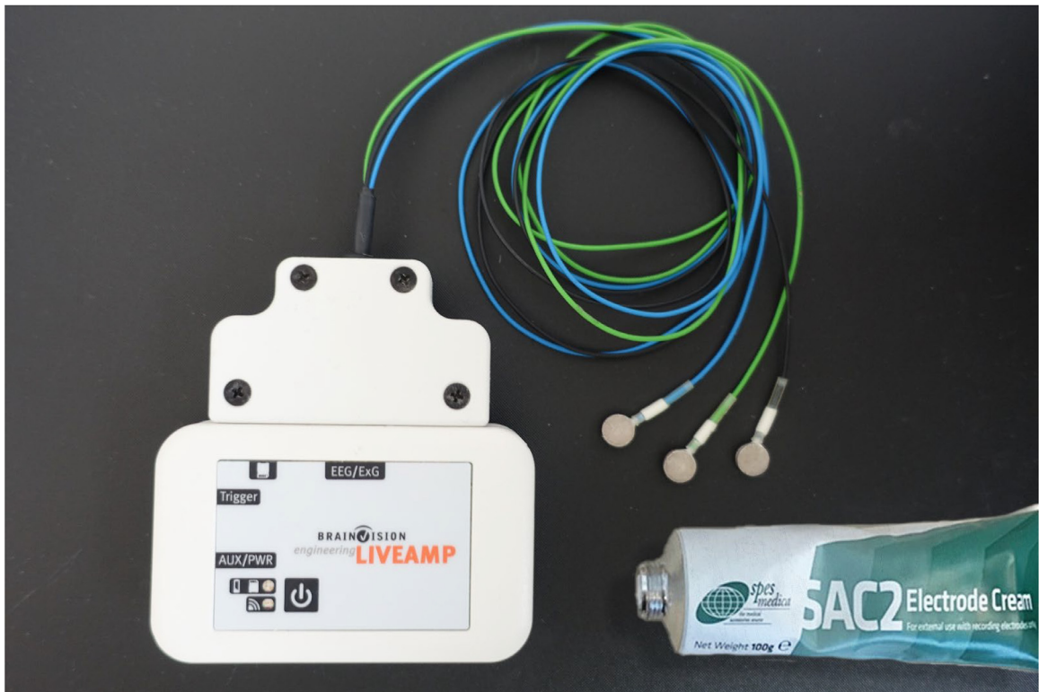
Fig. 1. Mobile EEG (LiveAmp), Electrodes (8 mm diameter) and electrode creme (SAC2 Electrode Cream).
