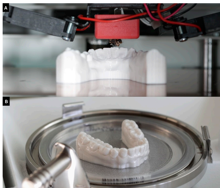
Figure 2. Printed FMD model on printing plate (A), model with thermoforming foil (B).
