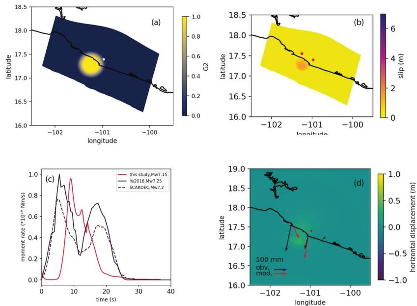
**Figure 7.** (a) Map view of the exponential function  $G_2$  which we use to prescribe the single asperity of Model B1. (b) Cumulative fault slip, (c) moment release rate, and (d) synthetic surface deformation of dynamic rupture Model B1 with a single asperity. The shown Global Positioning System stations are the same as in Figure 6b.
